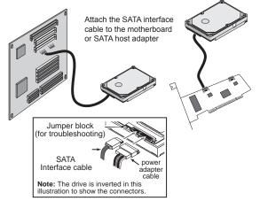
Note. Serial ATA connectors are keyed to ensure correct orientation.
