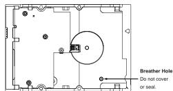
**Caution.** Do not cover, seal, or insert any object into this hole. If this hole is covered, sealed, or penetrated by any object, the drive reliability may be compromised and could lead to permanent damage and voids the warranty.
